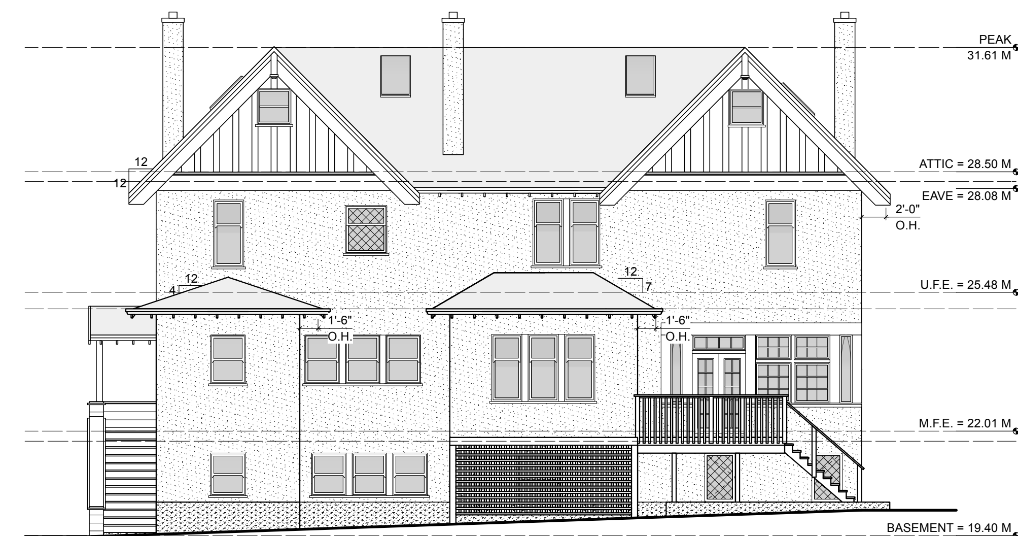
③ REAR (W) ELEVATION - EXISTING Scale: 1/8" = 1'-0"
