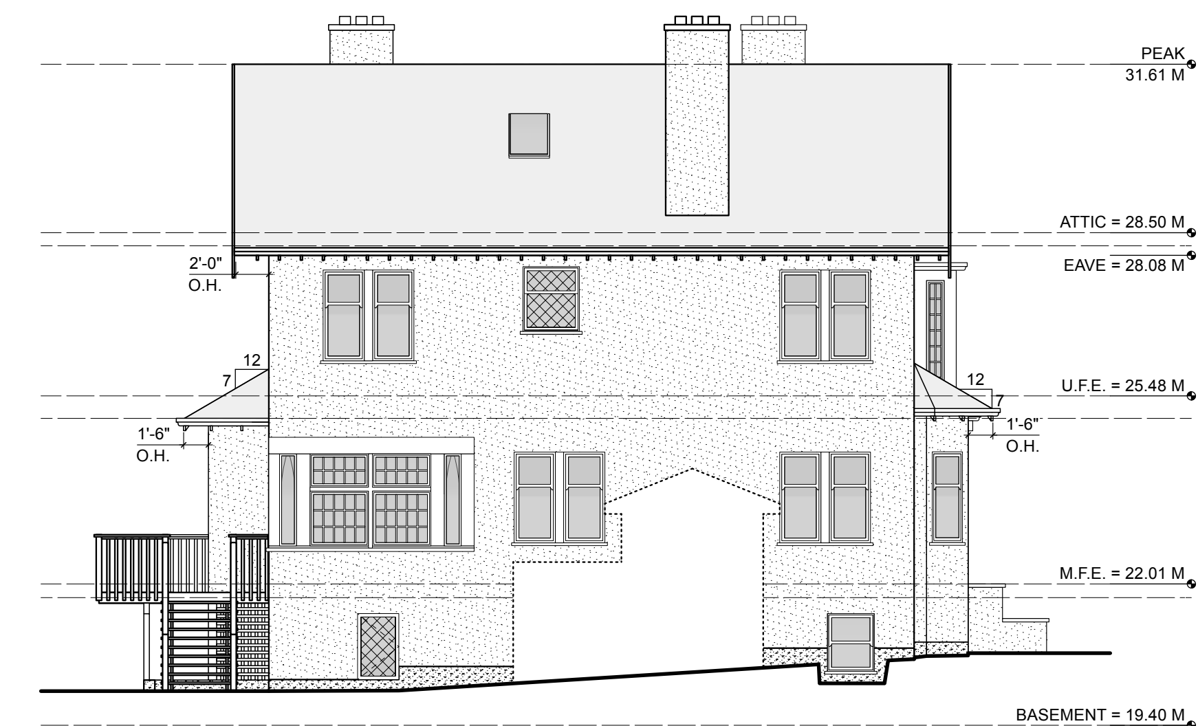
④ SIDE (S) ELEVATION - EXISTING Scale: 1/8" = 1'-0"
